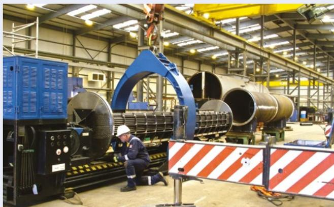
Unit Engineers & Constructors have cemented their long-standing relationship with Hadi Hamed Al Hamam Establishment with the supply of two 900 tube carbon steel tube bundles for a reactor feed and effluent exchangers in Saudi Arabia.
