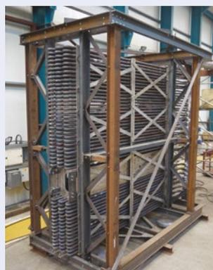
The replacement B601 superheater is for the site's Number One calciner unit waste heat boiler. Part of a larger order, this is the third time in recent years UEC has manufactured a superheater on this site and this project presented some challenges in production, particularly in the positioning and welding of 2¼ percent chrome panels to 1¼ chrome headers under braided preheat.
