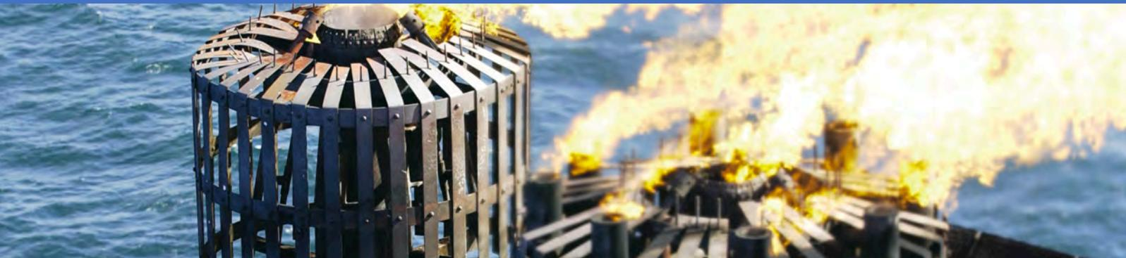
It is clear from the above tabulated data that our system offers an exceptionally high capture efficiency. Under normal, continuous conditions only 1.8% of the original flare gas flow is sent to the flare stack, resulting in an impressive 98.2% reduction in emissions to atmosphere.
