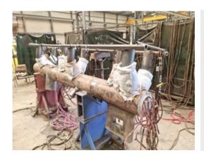
All manufacturing was completed at our main manufacturing facility in Swansea, South Wales. This included fabrication, pre heating by ceramic braids, post weld heat treatment utilising our in-house gas fired furnace, in house NDT and finally hydrostatic testing to 8000 psi.
